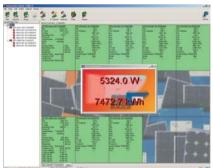
If required, the PC can also be connected with the Sunny Boy Control via modem. By connecting several Sunny Boy Controls, it is possible to monitor large scale plants with more than 50 Sunny Boys or Sunny Mini Centrals.
