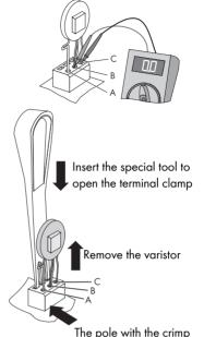
must be fitted to terminal A
