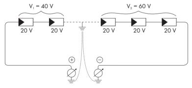
The ground fault is between the second and third module in this case.
