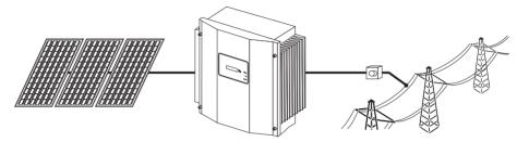
The Sunny Boy may only be operated with PV generators (modules and cabling) of protection class II. Do not connect any sources of energy other than PV modules to the Sunny Boy.
